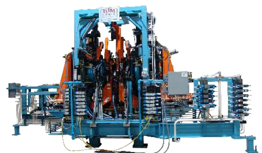
This large custom-built machine was designed to pierce and insert Spac® nuts in an automotive front cradle assembly.
