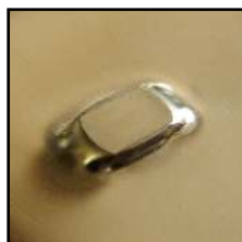
Die Side of completed joint
