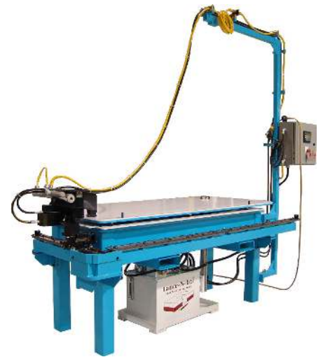
This custom solution uses a BTM 7006 handheld unit, fixed to a track to easily clinch various locations of a part.
