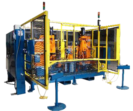
This custom dual workstation machine uses Tog-L-Loc® to assemble an automotive part.
