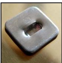
Punch Side of completed joint
